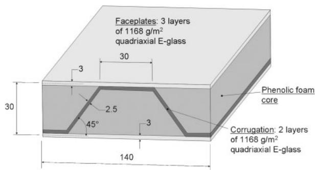
2 Geometry of panel tested in experimental programme, mm
