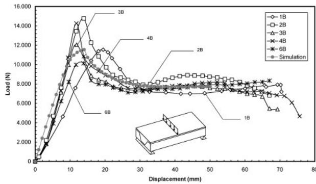
4 Three-point bending tests: load-deflection curve of z-core sandwich panels (B configuration)
