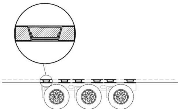
8 Sketch of design concept for structural floor of semi-trailer with corrugated core and metallic inserts for connection of composite floor to underframe
