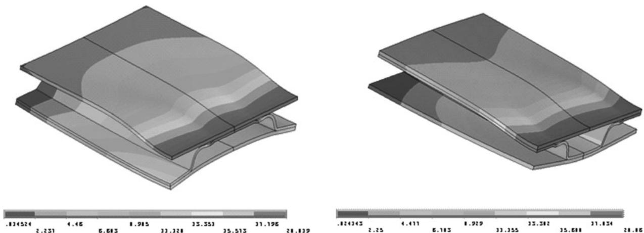
7 Deformation of composite layers in panel during bending test, A configuration (left) and B configuration (right)
