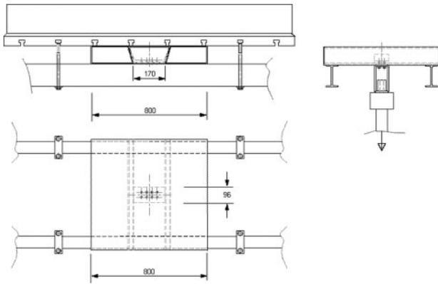
10 Schematic of test condition corresponding to composite panel (800×800 mm) supported by two metallic I beams transversal to corrugation direction and with insert at centre
