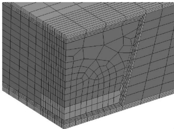
16 Finite element model of joint with rectangular insert and detailed view
