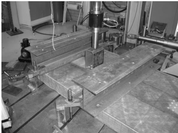
11 Test section mounted in test rig for flexural test
