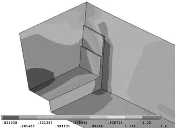
21 Equivalent stress distribution in foam around insert corresponding to 15 mm of applied displacement, MPa
