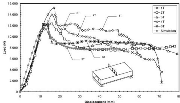
3 Three-point bending tests: load–deflection curve of z-core sandwich panels (A configuration)
