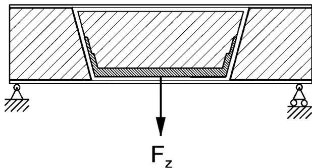
9 Schematic of three-point flexural test
