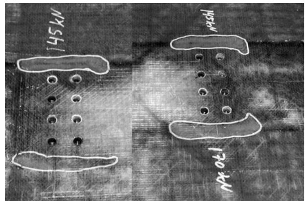
14 Details of extension of delaminations at surface of composite floor in correspondence to insert position
