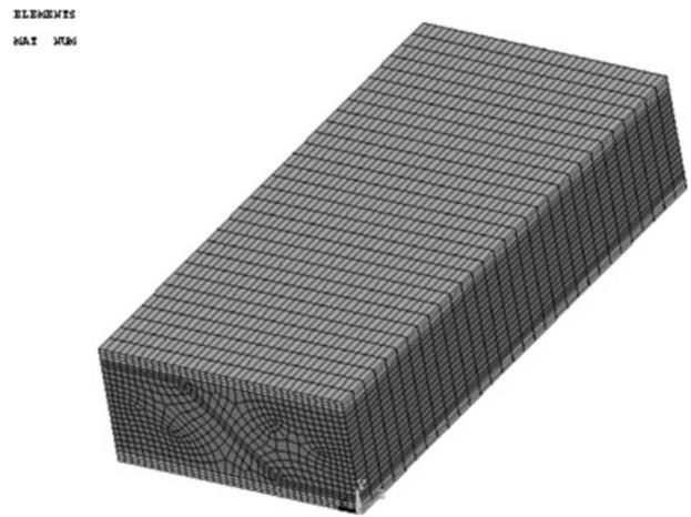
5 Finite element model of z-core panel for simulation of three-point bending tests (one-fourth of panel is modelled for symmetry)
