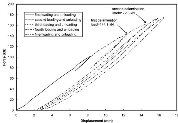
12 Flexural test on first prototype of composite floor with five loading and unloading cycles: first delamination occurring in correspondence of joint at ~144 kN of loading; second delamination at ~172.8 kN
