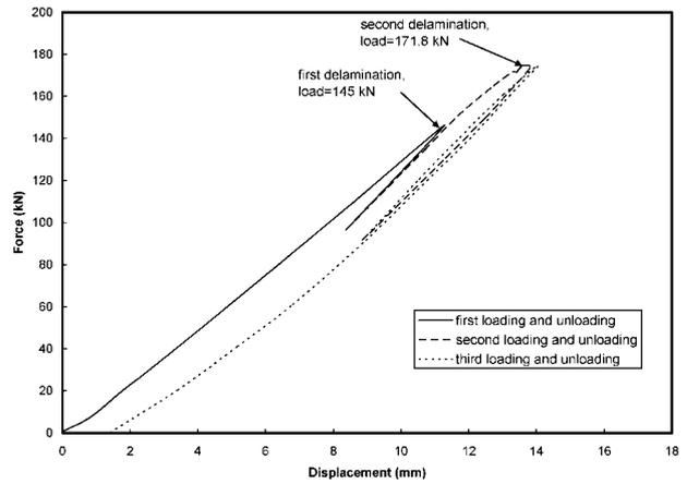
13 Results of flexural test on second prototype of composite floor, with first delamination occurring at 145 kN of loading and second delamination at 171.8 kN
