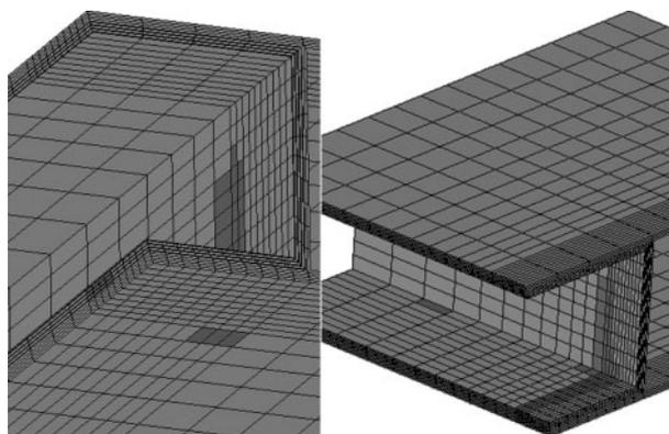
18 Localisation of areas of possible failure due to delamination
