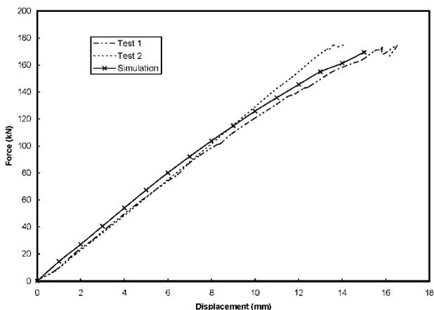
17 Results of simulation of flexural test and comparison with experimental curves
