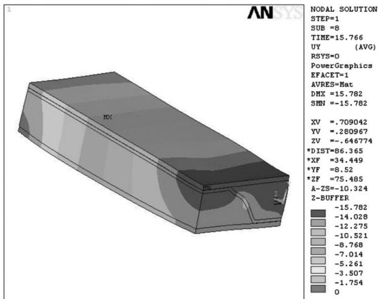
6 Distribution of displacements in panel bending analysis: imposed displacement of 20 mm distribution of total displacements, mm
