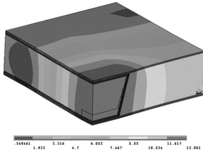
19 Sum of displacements corresponding to 13 mm of applied displacement, mm
