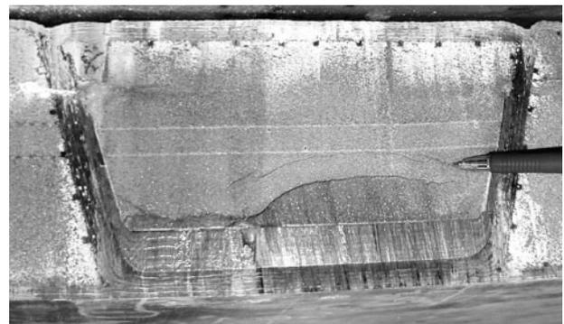
15 Section of sample after testing showing failure of foam above metallic insert
