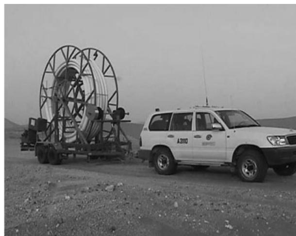
4 Flexibility of RTP permits coiling on drum: continuous lengths, up to 1 km between joints, may be deployed (or retrieved) by this simple means (Courtesy of Technip and Petroleum Directorate Oman)
