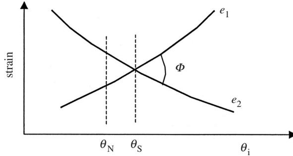
Figure 2. Relation between strain components and  $\theta_i$ . In a laminate, the stable angle of inclination  $\theta_S$  is not equal to  $\theta_N$ .
