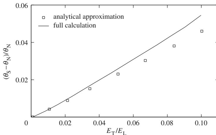
Figure 3. Deviation of the laminate stable angle from  $\theta_N$  as a function of  $E_T/E_L$ . The analytical approximation is given in (3.5).
