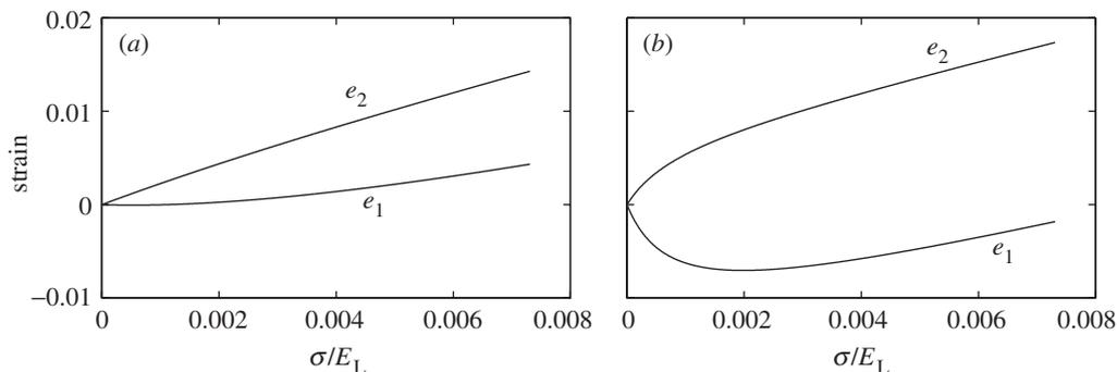
Figure 6. Effect of the ratio  $E_T/E_L$  on the stress–strain relations with a larger deviation,  $(\theta_S - \theta_i) = 0.01\theta_N$ , of the initial fibre inclination from the stable angle. (a)  $E_T/E_L = 10^{-2}$ . (b)  $E_T/E_L = 10^{-3}$ .
