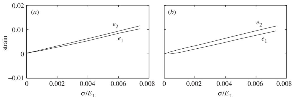
Figure 5. Effect of the ratio  $E_T/E_L$  on the stress–strain relations with a small deviation,  $(\theta_S - \theta_i) = 0.001\theta_N$ , of the initial fibre inclination from the stable angle. (a)  $E_T/E_L = 10^{-2}$ . (b)  $E_T/E_L = 10^{-3}$ .
