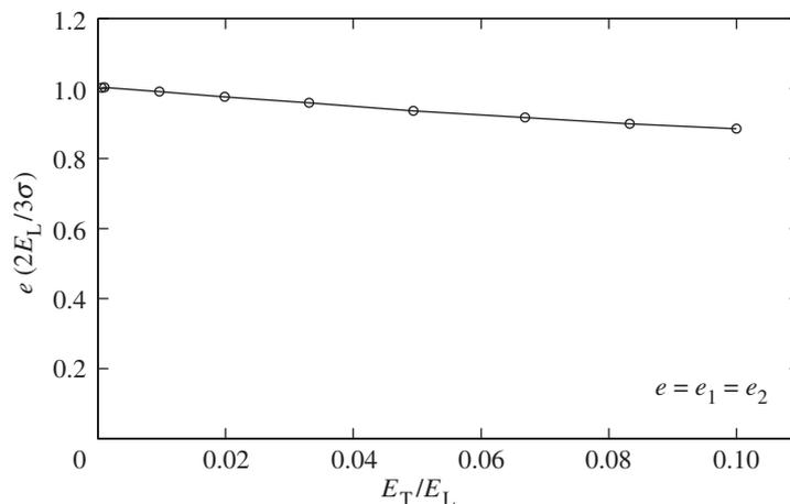
Figure 4. Strain at the stable angle as a function of  $E_T/E_L$ .
