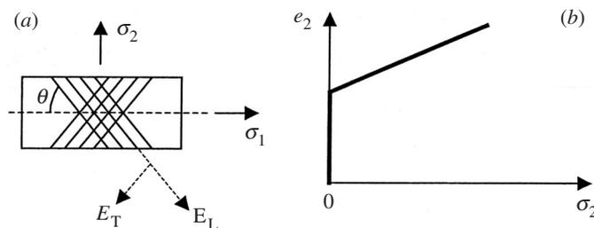
Figure 1. (a) Fibre orientation and applied stress. (b) Schematic of the stress–strain relation according to netting analysis when the fibres are not initially inclined at the ideal angle  $\theta_N = \pm \arctan \sqrt{2}$ . The fibres rotate at infinitesimal stress with increasing strain until they are inclined at  $\theta_N$ .
