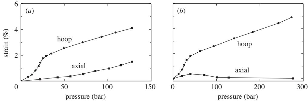
Figure 7. Examples of strain versus pressure in two thermoplastic reinforced pipes ((a) pipe A and (b) pipe B) supplied by two different manufacturers (after Chapman 1999).
