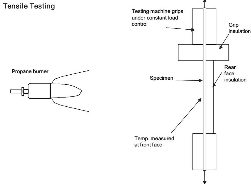
**Figure 4.** Experimental set-up for fire exposure under tensile load using a calibrated propane burner.
