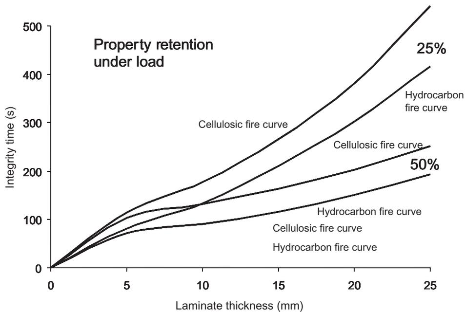
**Figure 20.** Predicted times for 50 and 25% retention of integrity under load for generic composite laminates. Type of fire exposure: 'cellulosic' and 'hydrocarbon' fire curves. Model assumes that failure mode is buckling and that property loss occurs when laminate reaches 170°C.
