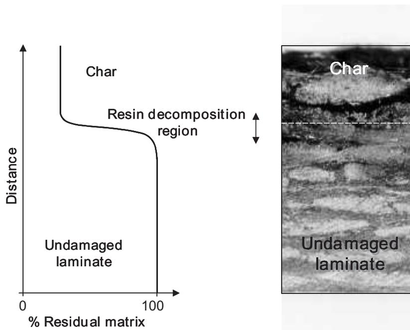
**Figure 2.** Schematic of resin degradation through laminate, with resin decomposition zone and residual char, alongside a cross-section through a glass/polyester woven roving laminate exposed to a heat flux of  $50 \text{ kW/m}^2$ .
