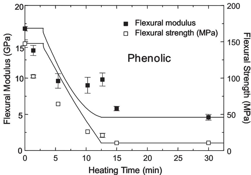
**Figure 15.** Change in residual flexural properties of glass-phenolic laminate with heating time at a heat flux of  $50 \text{ kW/m}^2$  (experimental points). The curves show the theoretical post-fire properties determined using the two-layer model.
