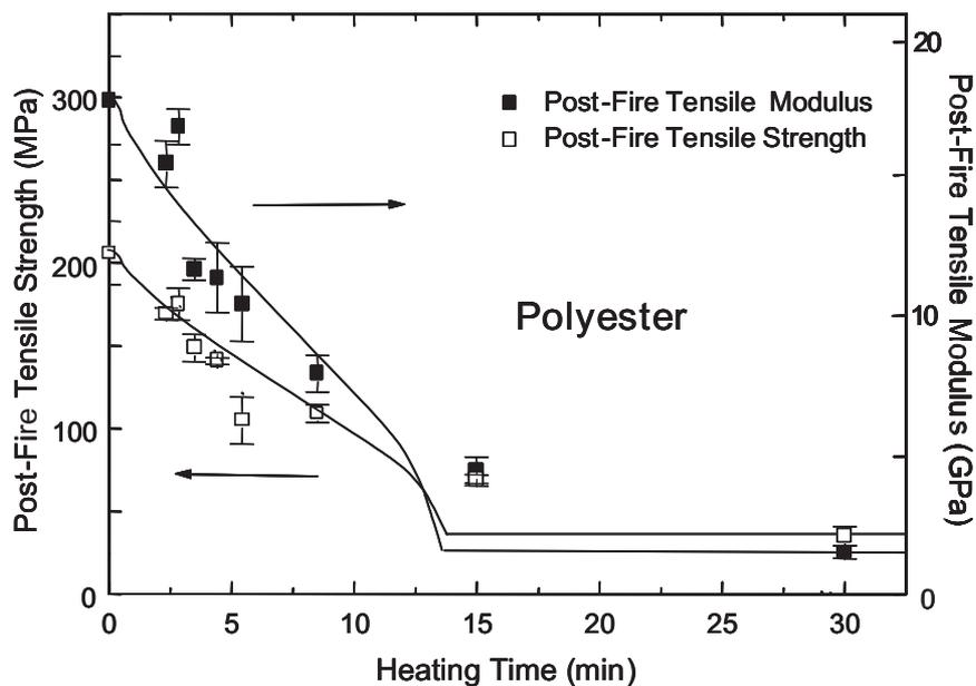
**Figure 11.** Change in residual tensile properties of glass–polyester laminate with heating time at a heat flux of  $50 \text{ kW/m}^2$  (experimental points). The curves show the theoretical post-fire properties determined using the two-layer model.
