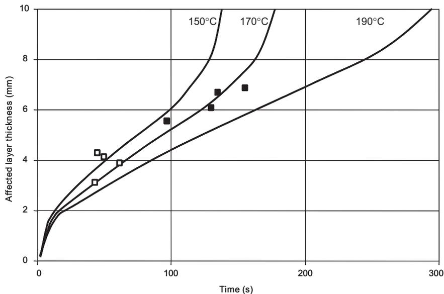
**Figure 17.** Relationship between thickness of heat-affected layer and time for 10-mm polyester laminates, subject to compressive loading and  $75 \text{ kW/m}^2$  heat flux. Experimental points are derived from the results shown in Figure 16. Open symbols: Euler buckling. Closed symbols: local buckling in the 'Boeing' test. Curves are from thermal model, assuming property loss to occur at 150, 170 and 190°C.
