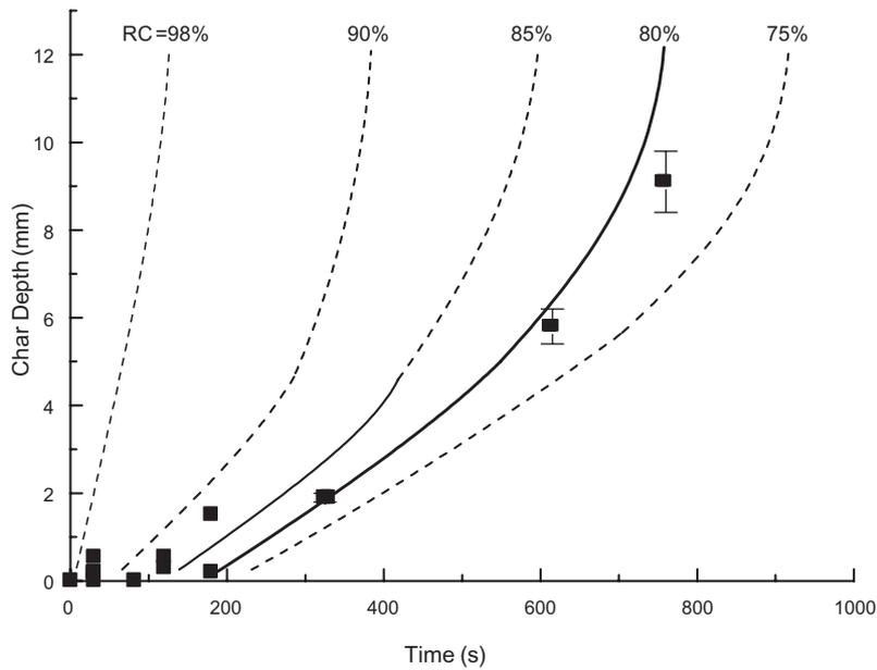
**Figure 9.** Thermal damage depth vs. heating time for a heat flux of  $50 \text{ kW/m}^2$  for 12-mm thick glass-phenolic laminates. The curves show the RRC at the interface between the char and undamaged laminate, determined using the thermal model, for RRC values in the range 75–98%.
