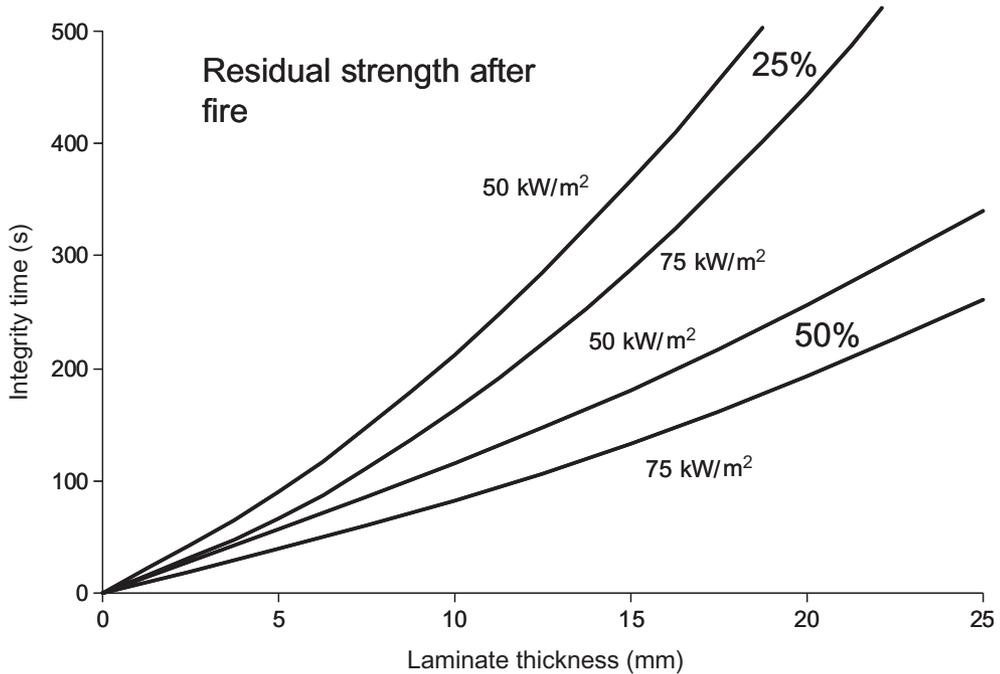
**Figure 21.** Predicted times for 50 and 25% retention of post-fire residual integrity for generic composite laminates. Type of fire exposure: 75 and 50 kW/m<sup>2</sup> constant heat flux. Model assumes that failure mode is buckling and that property loss occurs when laminate RRC reaches 80%.
