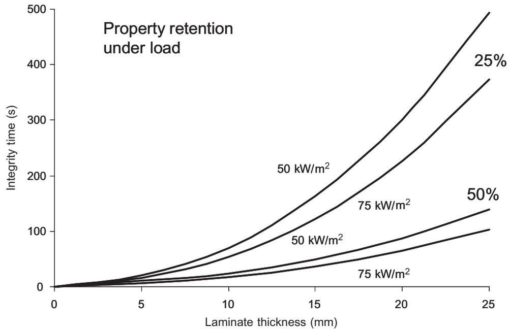
**Figure 19.** Predicted times for 50 and 25% retention of integrity under load for generic composite laminates. Type of fire exposure: 75 and 50 kW/m<sup>2</sup> constant heat flux. Model assumes that failure mode is buckling and that property loss occurs when laminate reaches 170°C.
