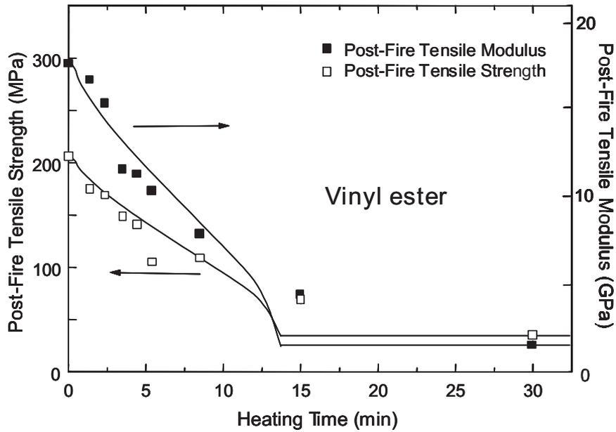
Figure 12. Change in residual tensile properties of glass-vinyl ester laminate with heating time at a heat flux of  $50 \text{ kW/m}^2$  (experimental points). The curves show the theoretical post-fire properties determined using the two-layer model.
