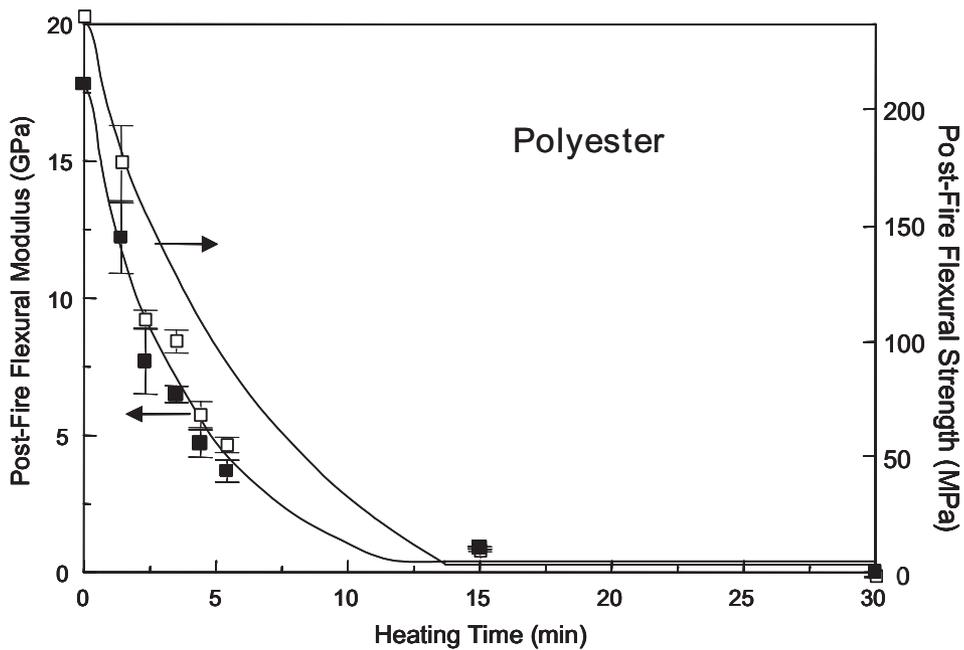
**Figure 14.** Change in residual flexural properties of glass-polyester laminate with heating time at a heat flux of  $50 \text{ kW/m}^2$  (experimental points). The curves show the theoretical post-fire properties determined using the two-layer model.
