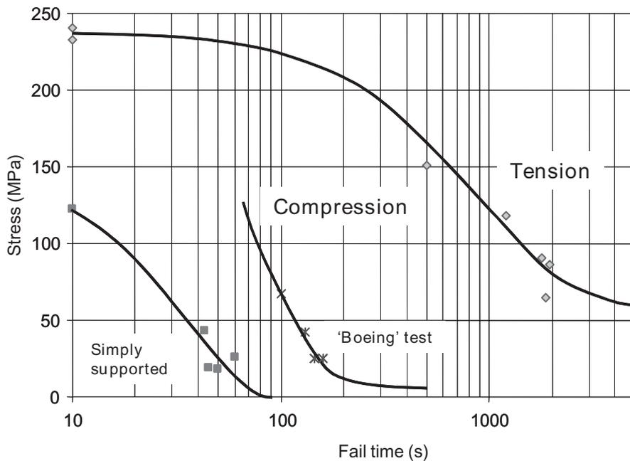
**Figure 16.** Relationship between stress and failure time for 10-mm polyester laminates, subject to  $75 \text{ kW/m}^2$  in burner test. Upper curve shows the results for tensile loading, middle curve shows compressive stress (Boeing compression jig,  $W/d = 10$ ), lower curve is compressive stress (Euler buckling,  $b/d = 15$ ).
