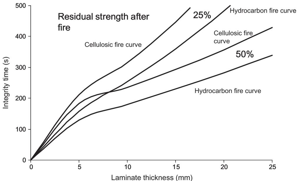
**Figure 22.** Predicted times for 50 and 25% retention of post-fire residual integrity for generic composite laminates. Type of fire exposure: 'cellulosic' and 'hydrocarbon' fire curves. Model assumes that failure mode is buckling and that property loss occurs when laminate RRC reaches 80%.
