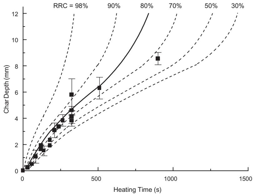
**Figure 7.** Thermal damage depth vs. heating time for a heat flux of  $50 \text{ kW/m}^2$ , for 12-mm thick glass–polyester laminates. The curves show the RRC at the interface between the char and undamaged laminate determined using the thermal model, for RRC values in the range 30–98%.
