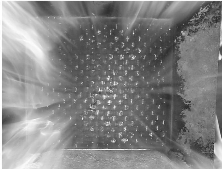
**Figure 5.** Above: experimental set-up for fire exposure under constrained compressive load using a calibrated propane burner. Below: sample under test.
