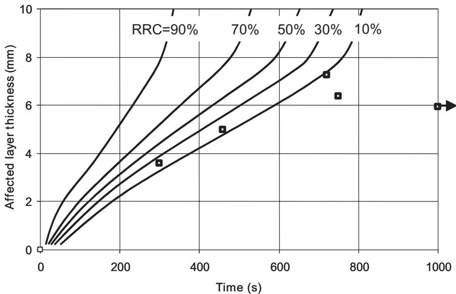
**Figure 18.** Relationship between thickness of heat-affected layer and time for 10-mm polyester laminates, subject to tensile loading and  $75 \text{ kW/m}^2$ . Experimental points are derived from the results shown in Figure 16. Curves are calculated from thermal model, assuming property loss to occur at RRC of 90, 70, 50, 30 and 10%.
