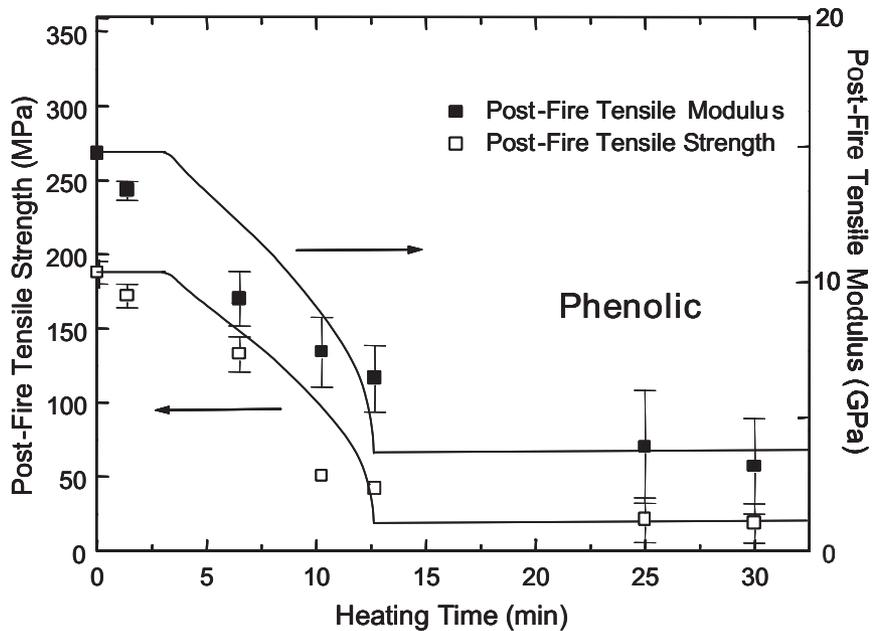
Figure 13. Change in residual flexural properties of glass-phenolic laminate with heating time at a heat flux of  $50 \text{ kW/m}^2$  (experimental points). The curves show the theoretical post-fire properties determined using the two-layer model.
