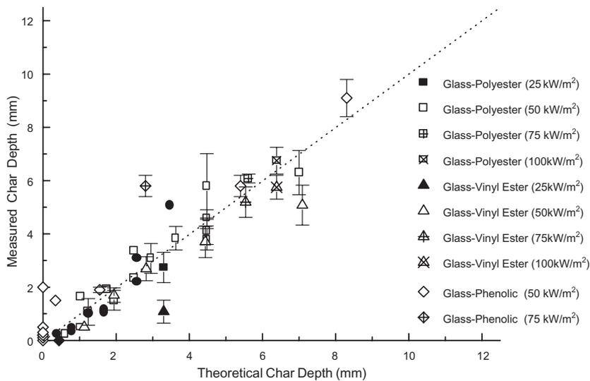
**Figure 10.** Comparison of the theoretical char depth, determined using the thermal model with char thickness values measured by microscopy, for all the laminate types studied at heat fluxes in the range 25–100  $\text{kW/m}^2$ .
