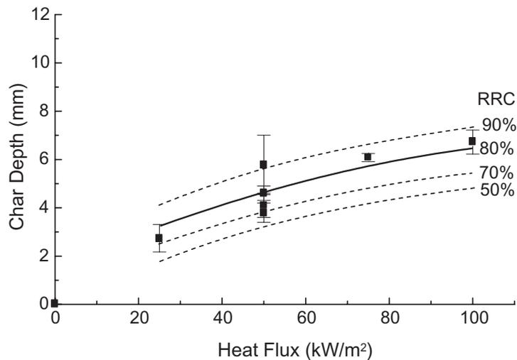
**Figure 8.** Effect of heat flux on char thickness for a heating time of 325 s for glass–polyester laminates. The curves show the RRC at the interface between the char and undamaged laminate determined using the thermal model.
