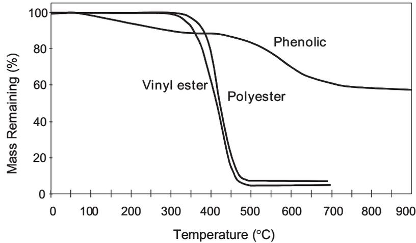
**Figure 6.** TGA curves at 25°C/min for isophthalic polyester, vinyl ester and phenolic resins in a nitrogen atmosphere.
