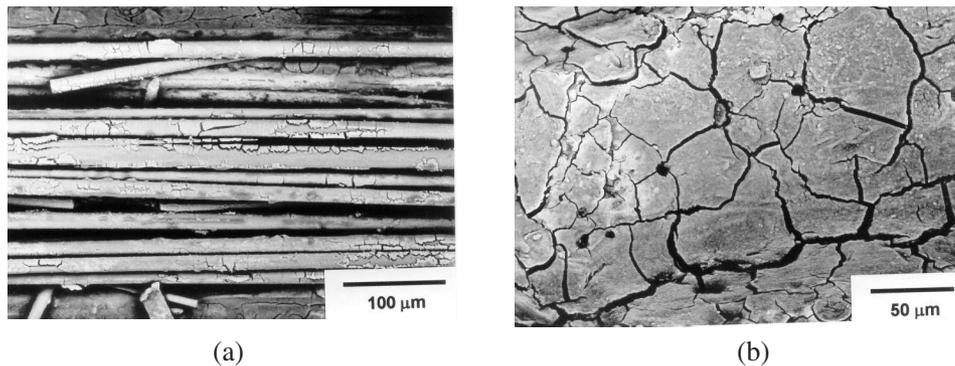
**Figure 3.** Scanning electron micrographs showing the microstructure of char in (a) glass–polyester and (b) glass–phenolic laminates. The char observed in glass–vinyl ester laminates is very similar to that in (a).
