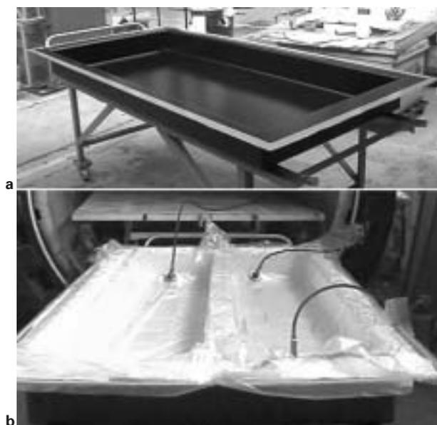
3 Tooling for battery tray, made from composite with cyanate ester matrix (ACG), and bagged component prior to processing
