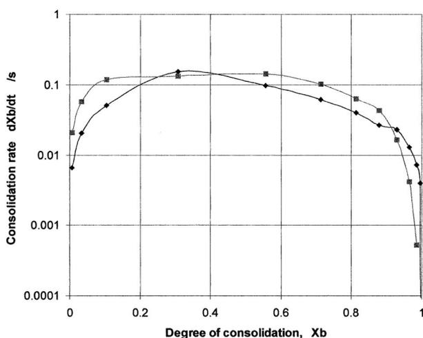
10 Calculated (squares) and measured (diamonds) values of the overall consolidation rate in process B, as function of consolidation during process run of Fig. 7
