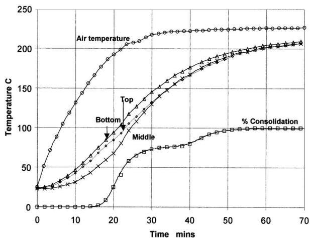
open symbols – experimental data; continuous line – consolidation model, using parameters in Table 2
