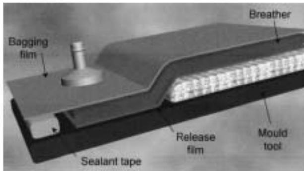
2 Schematic diagram showing bagging components prior to processing
