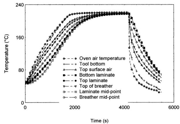
4 Thermocouple outputs during Comfil processing cycle for thermoplastic composite with copolyester matrix
