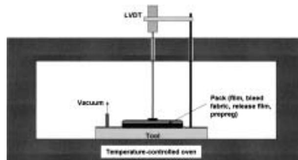
6 LDVT probe for measuring consolidation during processing
