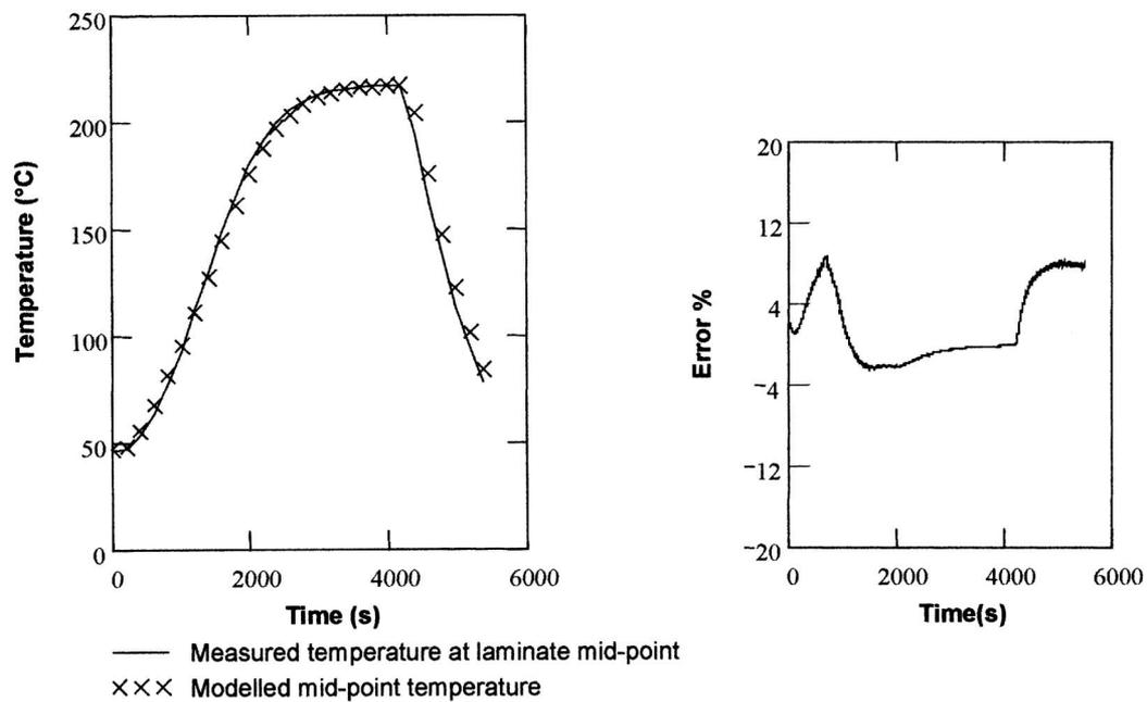
5 Comparison of measured laminate centreline temperature during process cycle (from Fig. 4) with values calculated from oven temperature profile, modelled using single point thermal values
