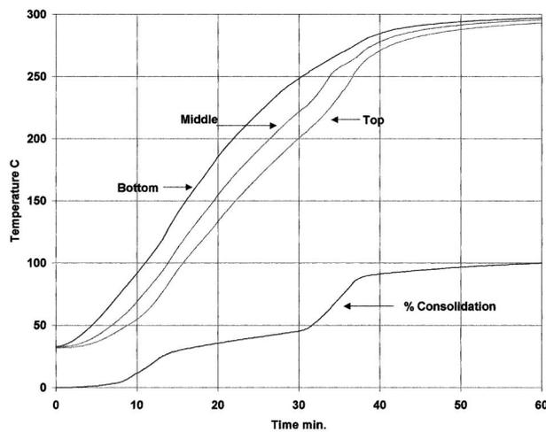
11 Processing cycle for Comfil PET homopolymer, showing temperature in oven air and in top, middle and bottom of moulding pack; percentage consolidation also shown
