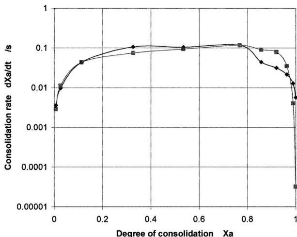
9 Calculated (squares) and measured (diamonds) values of overall consolidation rate in process A, as function of consolidation during process run of Fig. 7
